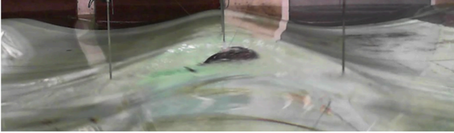
Fig. 12. Incident waves and ring wave at the sphere model in R12 for Setup 3 without reflective markers.
